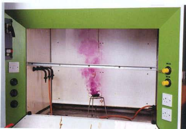
Figure 8.14 When solid iodine is heated it sublimes to form a gas. This is always done in a fume cupboard.
