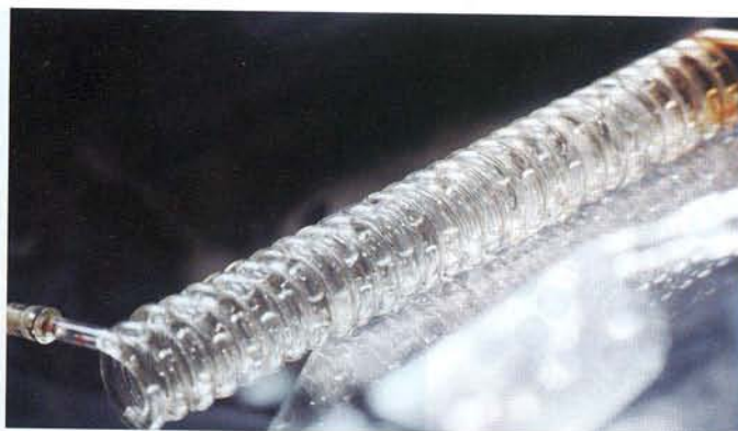
Figure 8.13 Steam passing through this condenser has cooled and condensed to form water.
