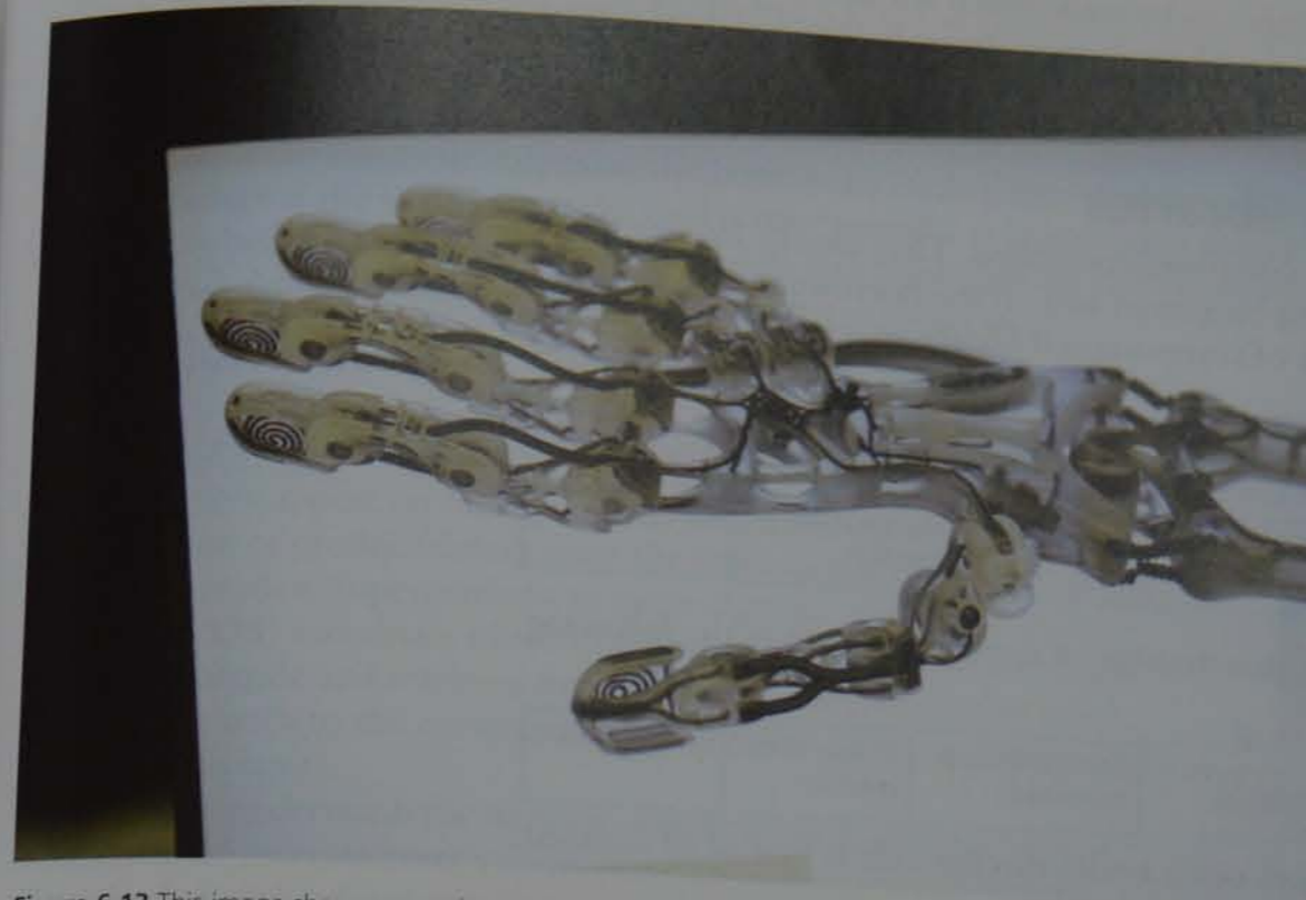
Figure 6.13 This image shows a prosthetic arm produced by a 3-D printer. Whilst the technology may not be cutting-edge, it can be life-changing to an amputee.
